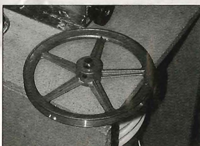
Figure 3: This nine-inch sheave was adapted with a copper bushing for proper mounting on the mill shaft.
